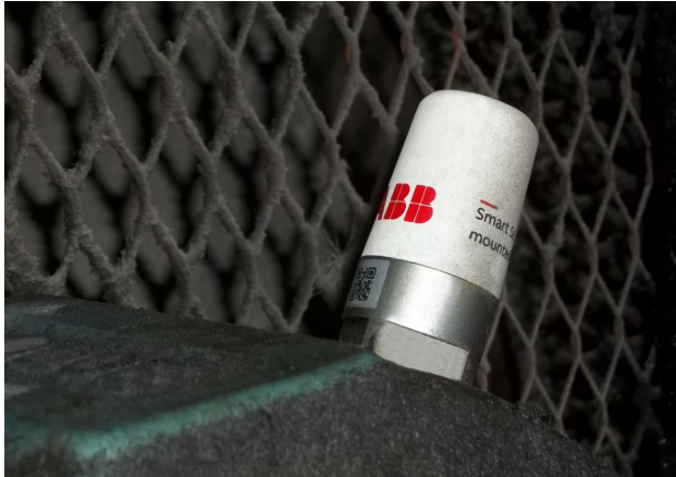
Caption: Transcontinental Advanced Coatings is using ABB Ability™ smart sensors on motors and mounted bearings to achieve zero downtime of critical equipment
